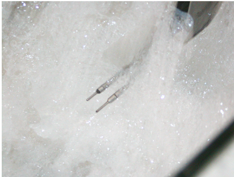
Fig. 2. Air–water flow measurements with two conductivity probes side-by-side. (A) Signal outputs in the shear layer of a hydraulic jump – transverse probe separation z = 11.5 mm, C = 0.156 , F = 136.7 Hz, y/d_1 = 0.91 , Fr_1 = 8.6 , d_1 = 0.024 m, x_1 = 1.0 m, x - x_1 = 0.2 m, W = 0.5 m. (B) Two probes separated by z = 10.5 mm, flow direction from bottom left to top right – local air–water flow properties: C = 0.79 , F = 20.6 Hz, y/d_1 = 4.15 , Fr_1 = 7.9 , d_1 = 0.024 m, x_1 = 1 m, x - x_1 = 0.2 m, W = 0.25 m.
